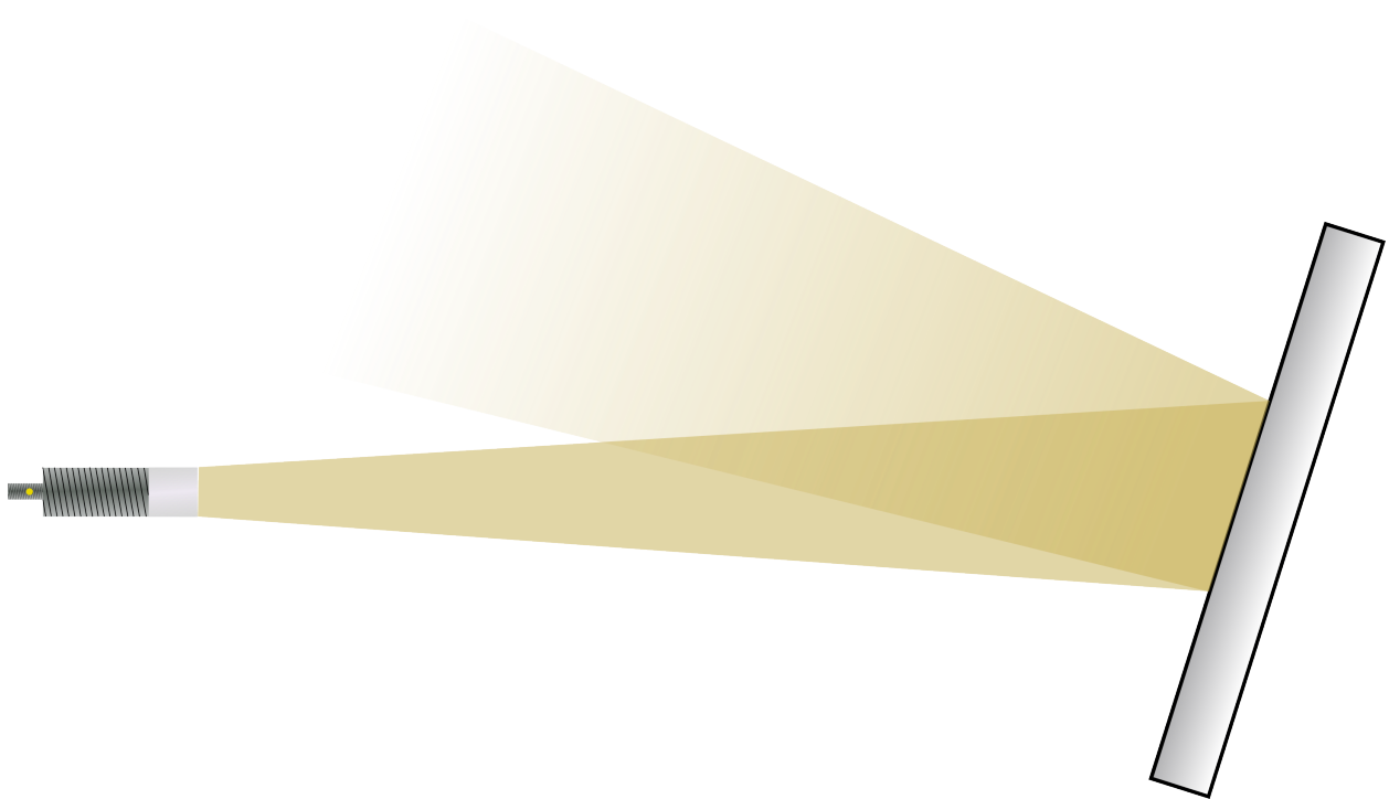
Fig. 7: Tilted planar target – Propagation of radar waves (schematic)
