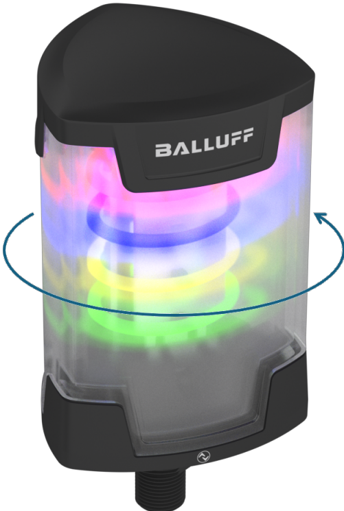
Fig. 14: Rotating beacon pattern
